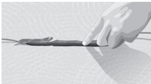
Fig. 3. Groove for joint of cold and heating cable
